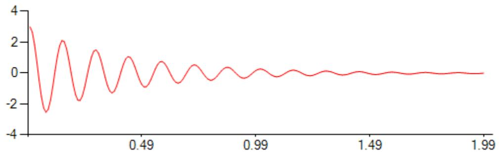
The amplitude of the system decays, this is why each peak is slightly less than the previous one.
