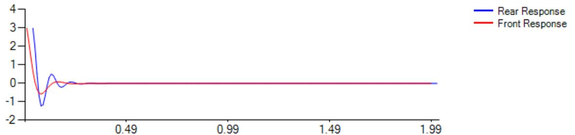
In this graph we can see that the rear catches up the front axle much faster, this is because the time constant of the rear response oscillator has decreased. However the rear axle now needs more damping because we increased the spring rate. If we increase the spring rate so that the front and rear axles have the same damping ratio, we get the following graph,
