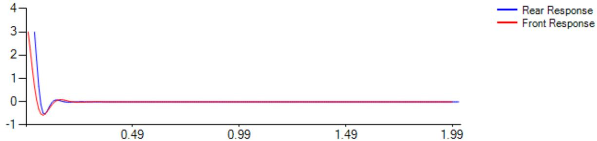
This is considered to be a good tune, the rear axle catches up the front, and the rear and front axles have the same damping ratio. This suspension setup would result in a car chassis that doesn't pitch, but heaves which is desirable.
