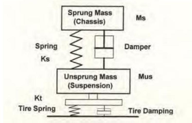
The system consists of two springs (Suspension Spring, Tire Spring) in series, and two dampers (Suspension Damper, and Tire Damper) in series.
