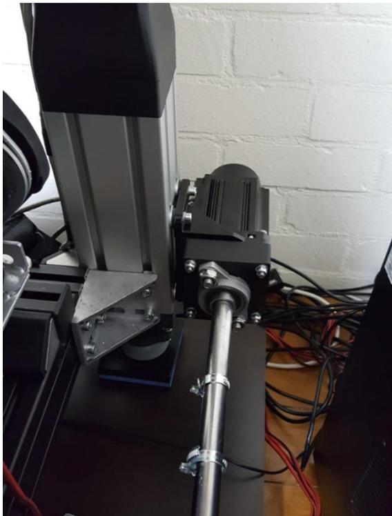
Mount the servo with the tube onto the extrusion. I have used big rings on the extrusion here, but that's not really needed. Do use the M6 rings onto the bolts.
