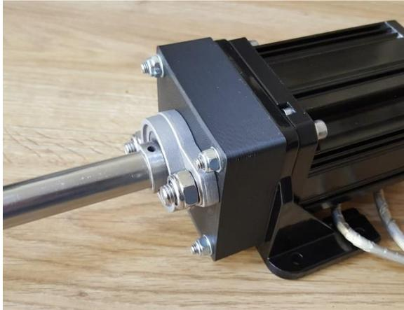
Place the M6 bolts with rings on both sides.
